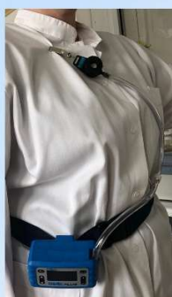
Figure 1. IOM Sampler and pump on worker (personal dosimetry).
