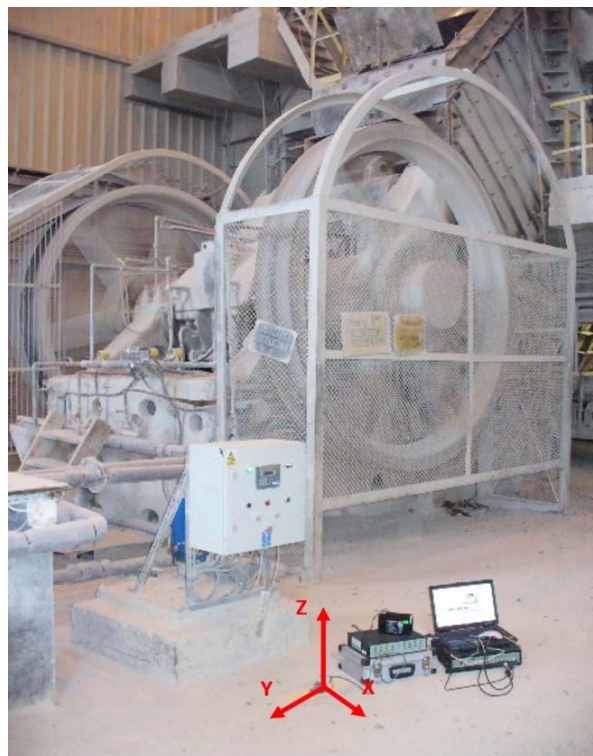
Figure 2. Location of measurement points and measurement directions at sample workstation (jaw crusher)
