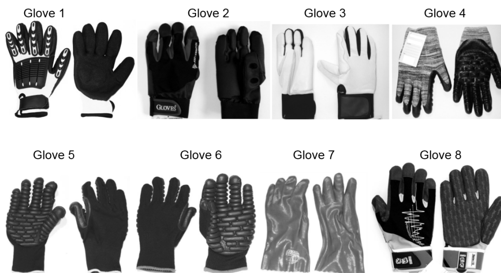
Figure 1. Anti-vibration gloves used for tests
