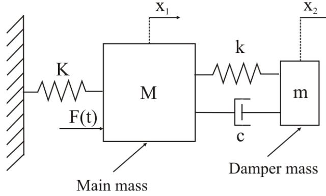
**Figure 4.** Dynamic model of TMD
