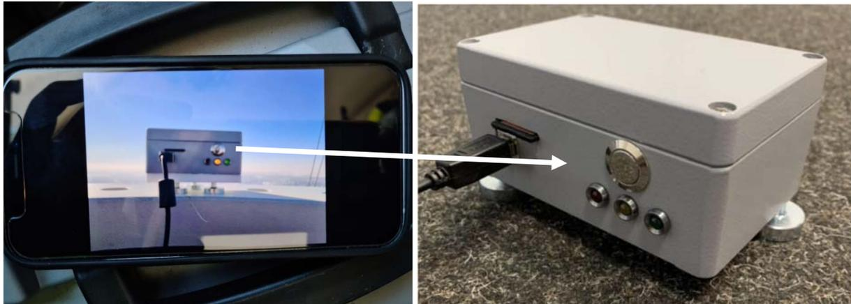
**Figure 7.** The Wireless transducer for vibration measurements
