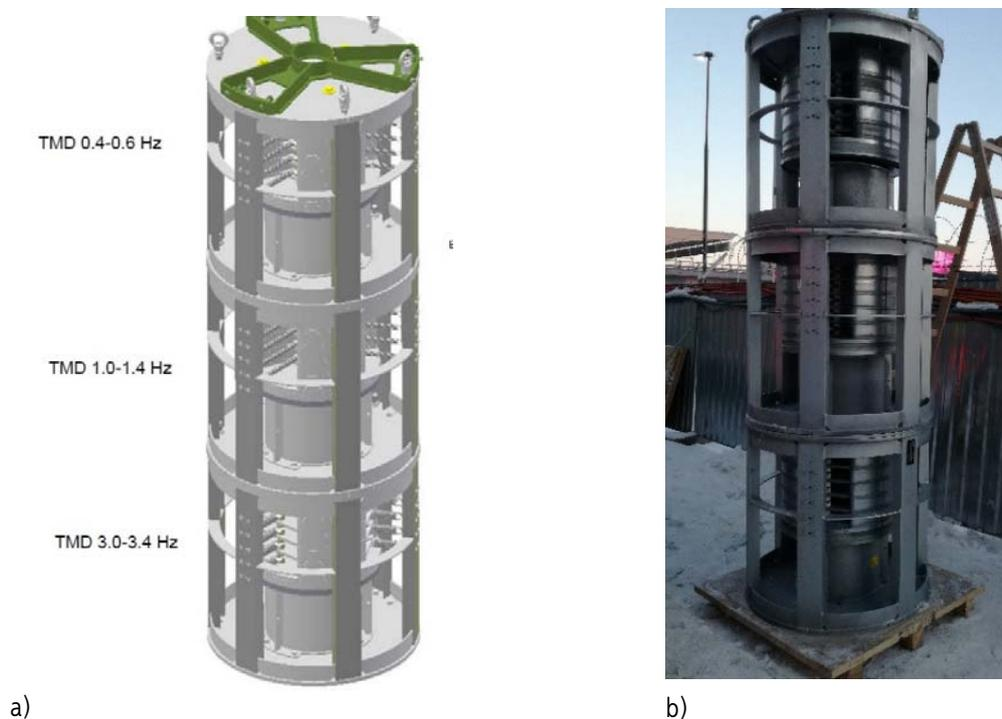
**Figure 6.** View of the TMD used in the spire; a) CAD model, b) photo
