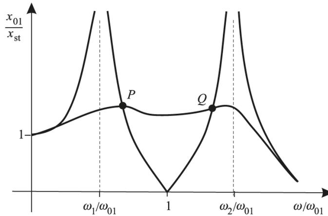
**Figure 5.** Vibration amplitude of the main mass
