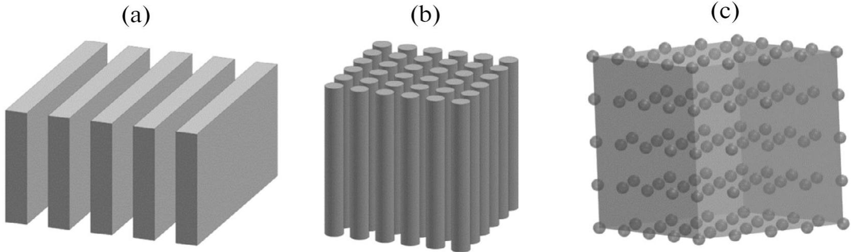
*(a) 1D sonic crystal consisting of plates arranged periodically;
