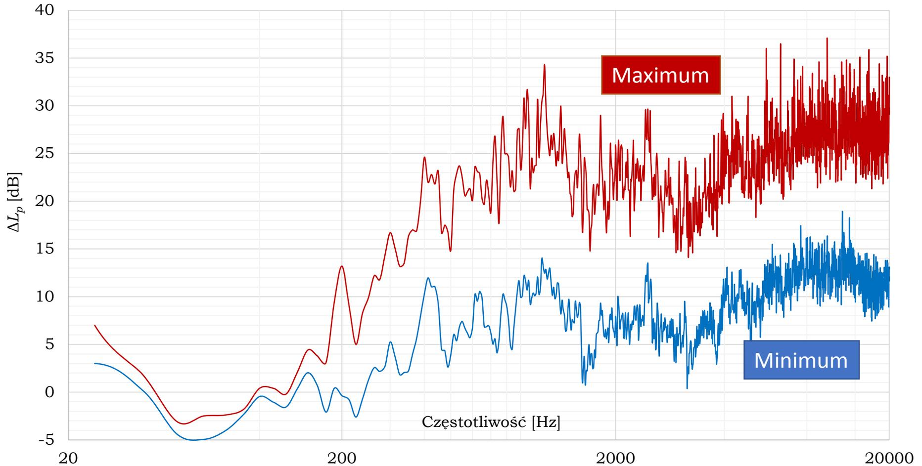
*Reduction of the sound pressure level at the measuring points*
