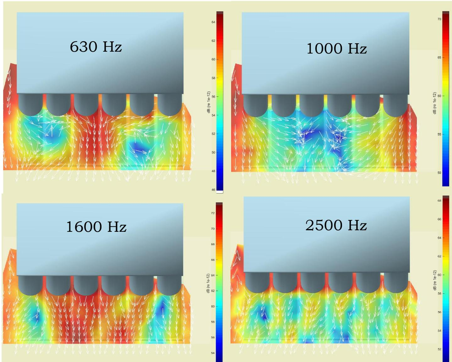
Distribution of the sound intensity vector in the horizontal measuring plane
