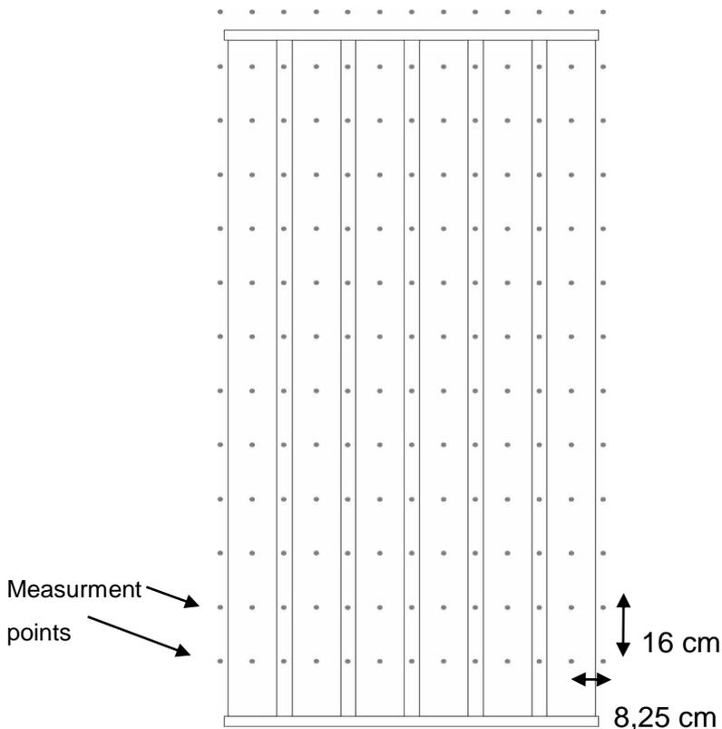
**Additional measurements** (with and without the barrier) of sound pressure level with the sound level meter (class 1) were carried out over 169 measurement points in vertical plane parallel to the barrier's surface with  $d_M = 0,25$  m.
