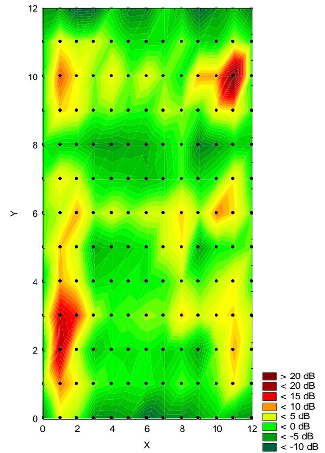
Distribution of the reduction of the sound pressure level at the measuring points
