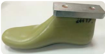
Rys. 2. Model „kopyta” stopy wg PN-EN ISO 13287:2013-04 Fig. 2. A „hoof” model of a foot according to PN-EN ISO 13287:2013-04
