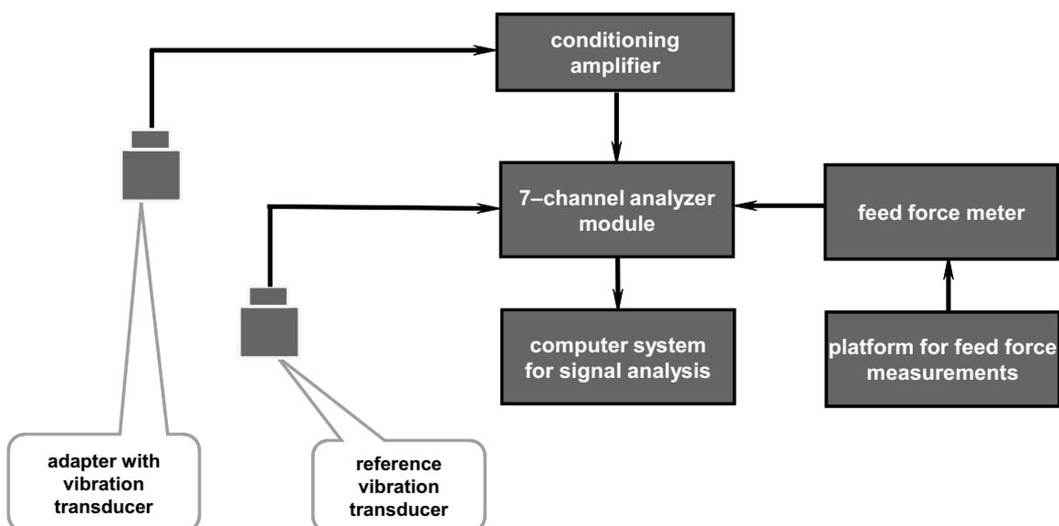
Figure 3. Measuring system for testing the vibration transmissibility of gloves.
