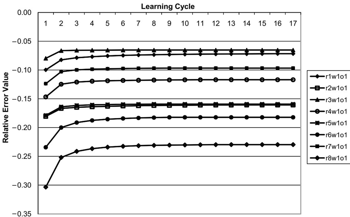
Figure 7. Changes in the value of the relative error when training a neural network simulating the behaviour of 8 gloves (r1–r8) for operator 1 (o1) using a drill (w1).
