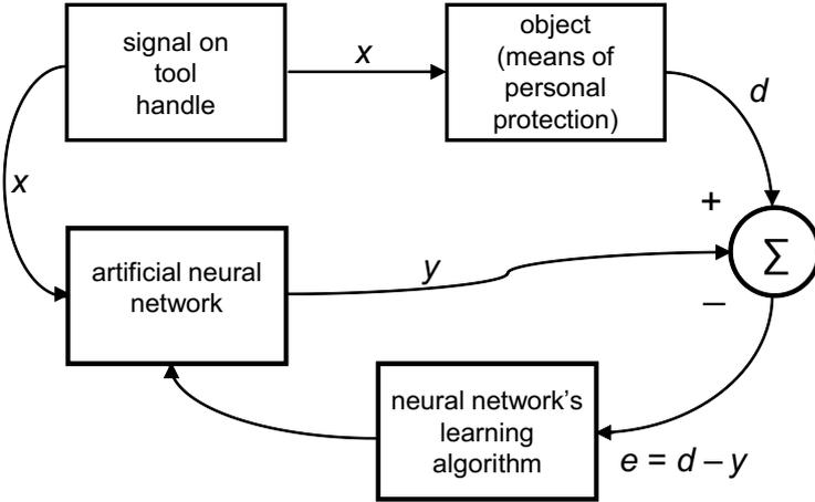
Figure 1. Identifying parameters of anti-vibration gloves with a neural network.
