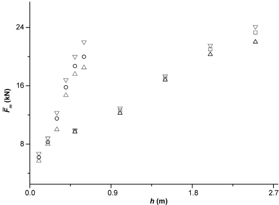
**Figure 9. Test results of adjustable lanyards.** Notes.  $\circ$ — $\bar{F}_m$  for lanyards made of steel wire rope with polyamide braid,  $\square$ — $\bar{F}_m$  for lanyards made of aramid rope,  $\triangle$ — $F_{m \min}$ ,  $\nabla$ — $F_{m \max}$ .
