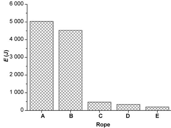
**Figure 4. Energy (transformed into elongation) generating in a rope of the initial length of  $L_0 = 2$  m a force of  $F = 20$  kN.** Notes. A—14-mm diameter three-strand polyamide rope, B—18-mm diameter three-strand polyamide rope, C—10-mm diameter aramid rope, D—12-mm diameter aramid rope, E—8-mm diameter steel wire rope.
