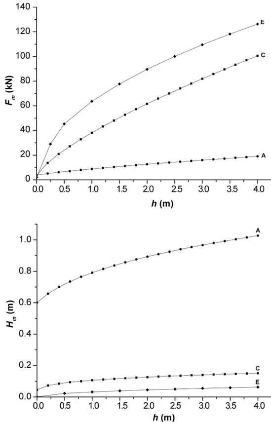
**Figure 8. The results of a numerical simulation.** Notes.  $F_m$ —maximum value of the force acting on the end of a lanyard,  $H_m$ —maximum value of the elongation of a lanyard; A—14-mm diameter three-strand polyamide rope, C—10-mm diameter aramid rope, E—8-mm diameter steel wire rope.
