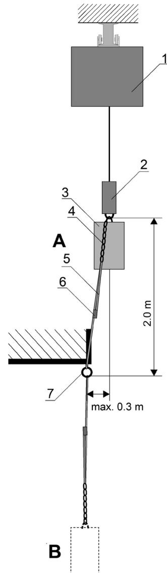
**Figure 6. Dynamic strength test for lanyards (according to EN 364:1992) [5].** Notes. A—situation before the test, B—situation after fall arrest, 1—power winch for lifting and lowering test mass, 2—quick release device, 3—test mass of 100 kg, 4—chain, 5—lanyard, 6—length adjuster of a lanyard, 7—anchor point.
