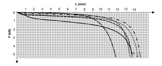
Figure 7. Characteristics of materials used for protective padding of helmets (samples 15 mm thick and 50 mm in diameter). *Notes.* 1—porous polyurethane, 2—foamed polystyrene of density 67kg/m³, 3—foamed polystyrene of density 29kg/m³, 4—foamed polystyrene of density 22kg/m³, 5—foamed polystyrene of density 13kg/m³, 6—microrubber.
