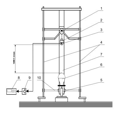
Figure 2. A stand for a shock absorption test of a helmet during side impact. *Notes.* 1—electromagnetic release device; 2—striker; 3—Endevco (type 7231C-750, USA) acceleration transducer; 4—guide poles; 5—mechanism fastening the headform; 6—headform; 7—bracket column; 8—Kikusui (type COM 7101A, Japan) digital oscilloscope with memory; 9—Endevco (type 106, USA) amplifier with an analog filter; 10—lifting truck for the striker.
