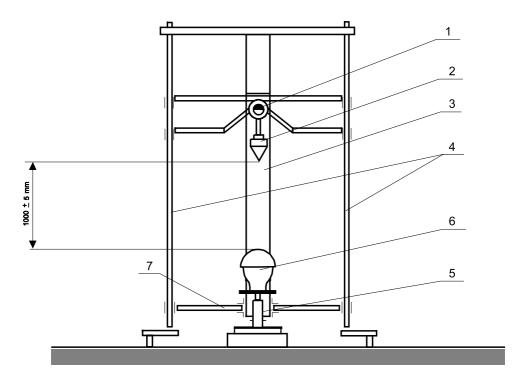
**Figure 4. A stand for a resistance to penetration test of a helmet during side impact.** *Notes.* 1—electromagnetic release device, 2—punch, 3—bracket column, 4—guide poles, 5—mechanism fastening the headform, 6—headform, 7—lifting truck for the punch.
