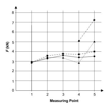
Figure 8. Shock absorption of a Prosna type protective helmet with protective padding made of foamed polystyrene. *Notes*. ×—at the top of the shell, O—from the front of the shell, □—from the back of the shell, △—from the side of the shell, ★—in the attachment plane.
