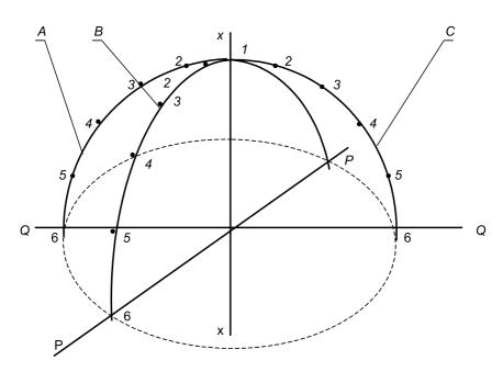
**Figure 1. Location of measurement points on the shell of a safety helmet.** *Notes.* x–x—axis resulting from the section of characteristic planes; 1QQ—symmetry plane of the head, 1PP—plane perpendicular to the symmetry plane of the head; A, B, C—curves resulting from the section of the shell of the helmet by two characteristic planes, along these curves the measurement points are located; 2–6—measurement points of the force.
