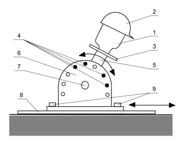
Figure 3. A diagram of a mechanism that enables an inclination of the headform at a given angle. *Notes.* 1—headform, 2—testing helmet, 3—plates that enable the rotation of the headform around the axis, 4—clamping screw, 5—rotated beam, 6—plates holding the beam, 7—rotation axis of the beam, 8—guide rail, 9—screws blocking displacement.
