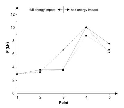
Figure 5. Maximal value of the force transmitted to the headform during impact in a Prosna type helmet. *Notes.* —front impact, —back impact, —side impact.
