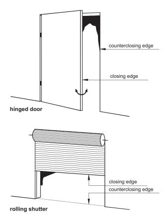
Figure 1. Crushing points between closing edge and counterclosing edge of doors and gates.
