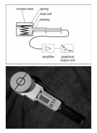
Figure 4. Measuring device for crushing forces.
