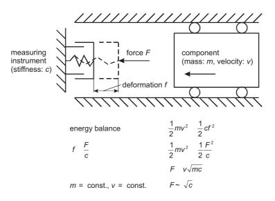
Figure 2. Influence of the measuring instrument's stiffness on the dynamic force.
