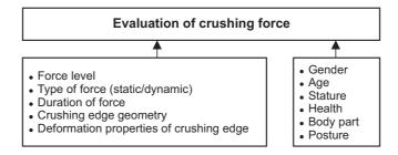
Figure 3. Examples of parameters to be considered in the evaluation of crushing forces.
