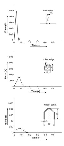
Figure 10. Crushing force versus time diagrams for different edges at uniform motor power.
