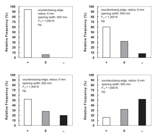
Figure 13. Sensory evaluation of dynamic forces from 1,000 to 1,600 N on the hip in a hinged door.
