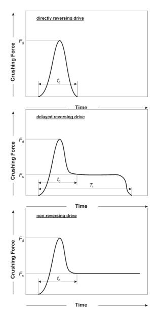
**Figure 9.** Characteristic crushing force-time diagrams. *Notes.*  $F_{d}$ —maximum dynamic force,  $F_{s}$ —static force,  $t_{d}$ —period of time during which the dynamic force acts,  $T_{t}$ —total duration of force application.
