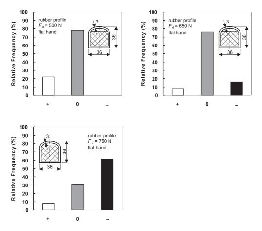
Figure 12. Sensory evaluation of dynamic forces from 500 to 750 N on the hand, held flat and extended, in a sliding door with an edge fitted with a rubber profile.
