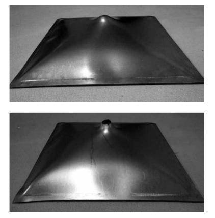
Figure 3. Bulging (top) and penetration (bottom) for steel sheet.
