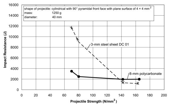
Figure 6. Impact resistance of polycarbonate and steel sheet using sharp ceramic projectiles of different strengths.
