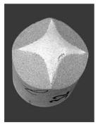
Figure 8. Ceramic projectile (strength: 80 N/mm<sup>2</sup>) with 90° pyramidal front face and  $4 \times 4$  mm plane surface after impact on steel sheet, projectile energy: 1381 J.
