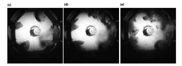
Figure 13. Grinding wheel fragments during impact on test samples.
