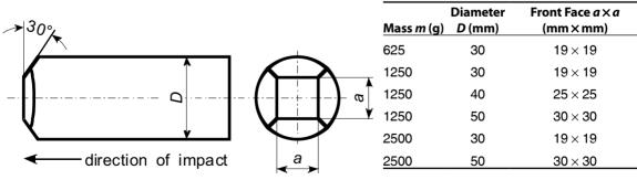
Figure 1. Steel projectiles (square-shaped front face).
