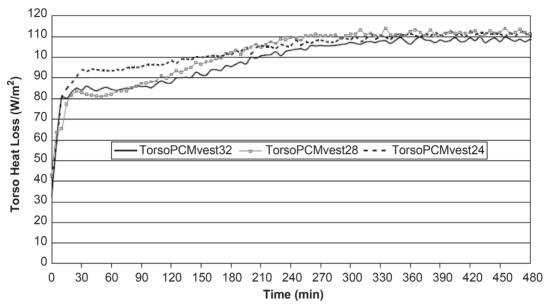
Figure 2. Heating effects of phase change material (PCM) vests ( $T_{\text{melt}}$  = 32, 28, and 24 °C) on the thermal manikin in the subzero environment [47].
