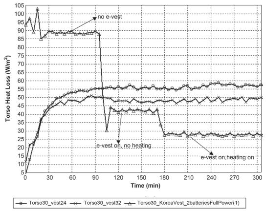
Figure 3. Manikin torso heat losses for phase change material (PCM) vests and electrical heating vest [34]. *Notes.* PCM vests worn over manikin stretch coverall,  $T_{\text{manikin}} = 30 \,^{\circ}\text{C}$ ,  $T_{\text{a}} = -4 \,^{\circ}\text{C}$ ,  $V_{\text{a}} = 0.4 \,\text{m/s}$ .
