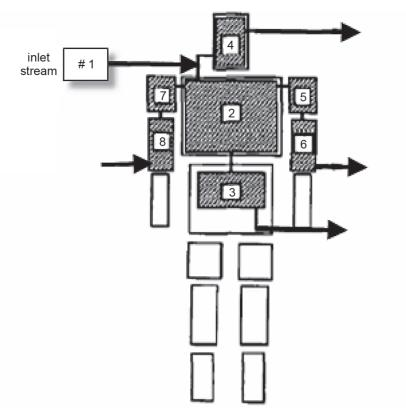
Figure 5. Schematic representation of heat exchanger elements and flow path used to form an airwarming vest [65].
