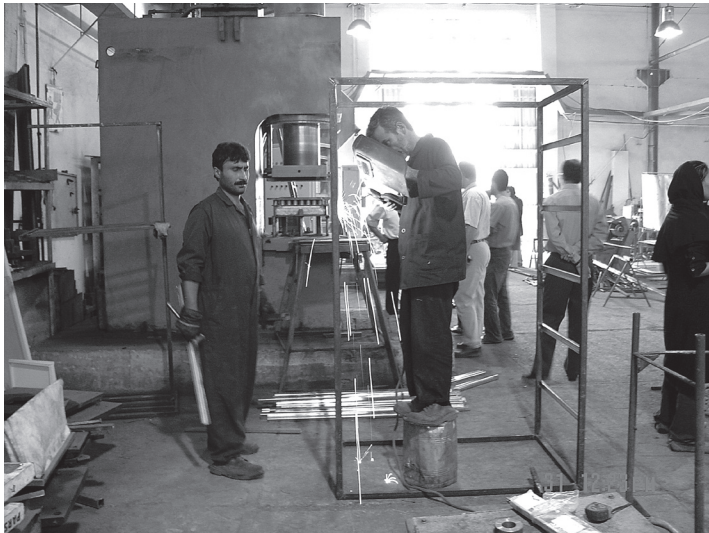
Figure 5. Worksite before improvement: no personal protective equipment for welder and coworkers, poor posture.
