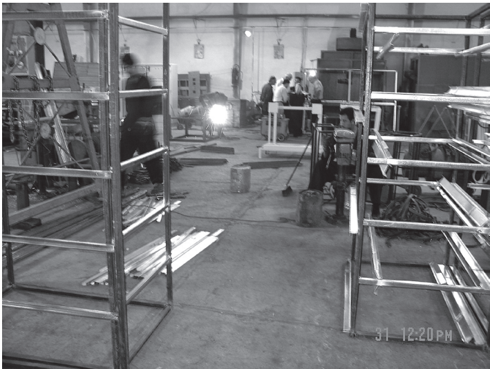
Figure 3. Worksite before improvement: no marked escape routes clear of obstacles, air pollution.
