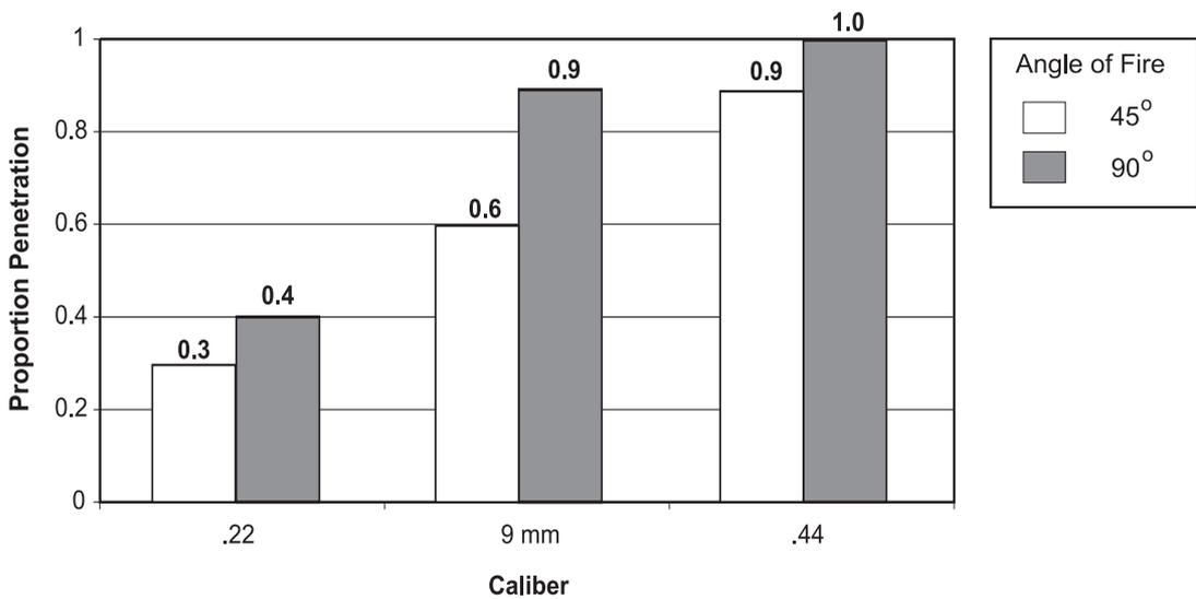
Figure 3. Comparison of caliber and angle of fire.
