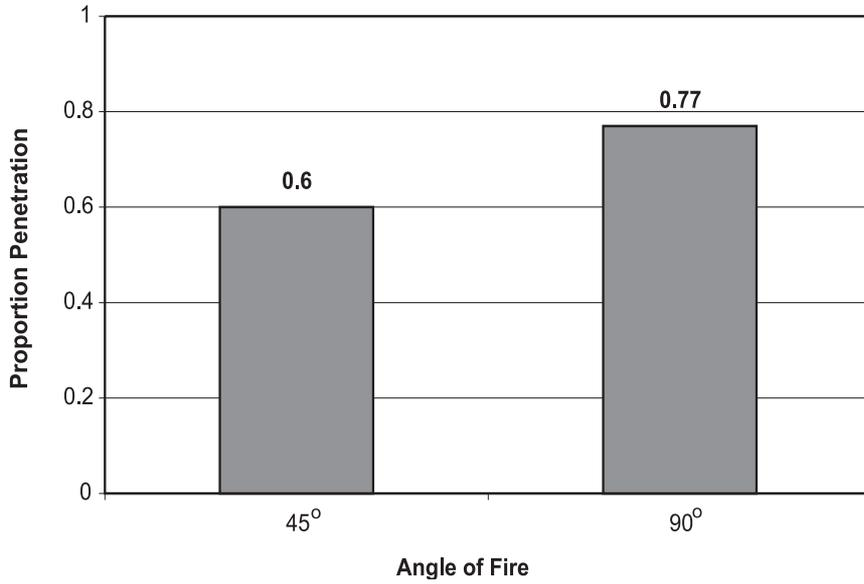
Figure 2. Comparison of the angle of fire and the associated proportion of penetration for each angle.
