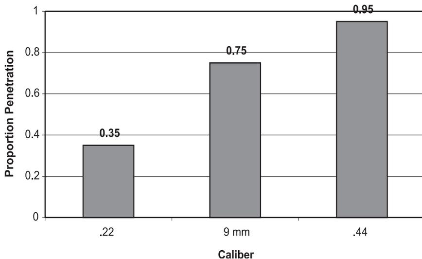
Figure 1. Comparison of the calibers and the associated proportion of penetration for each caliber.
