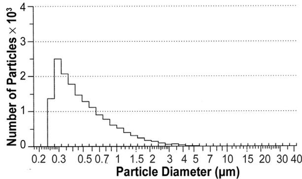
**Figure 4. Particle size distribution of metallurgic dust.** Notes. Geometric mean diameter ( $\mu\text{m}$ ) = 0.504, geometric standard deviation = 1.797.
