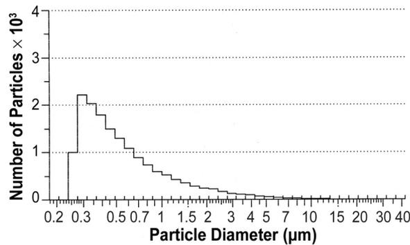
**Figure 3. Particle size distribution of coal dust.** Notes. Geometric mean diameter ( $\mu\text{m}$ ) = 0.563, geometric standard deviation = 2.010.
