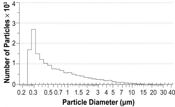
**Figure 2. Particle size distribution of copper-mine dust.** Notes. Geometric mean diameter ( $\mu\text{m}$ ) = 0.636, geometric standard deviation = 2.409.
