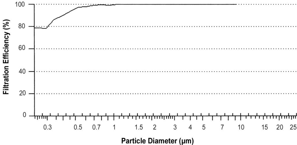
**Figure 13 Relationship between filtration efficiency (vertical axis) and aerosol particle diameter (horizontal axis) for melt-blown polypropylene filter material, electrified at 5 kV, and steelworks dust.**
