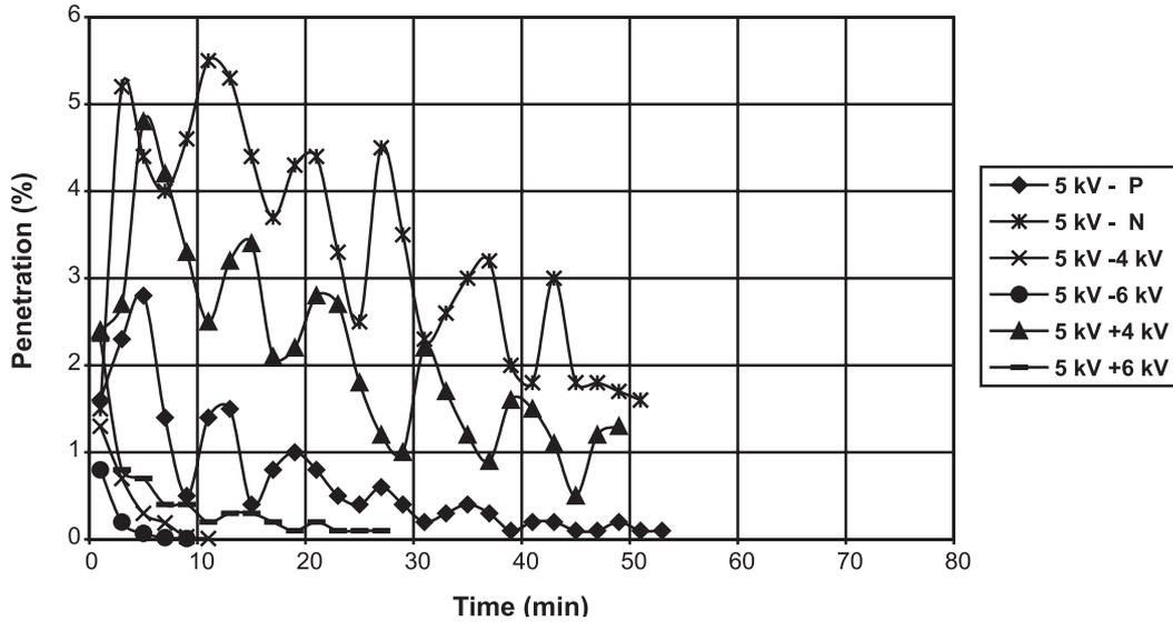
Figure 9. Changes in penetration with time of loading with coal dust (as specified by Standard No. PN-EN 143:2004 [10]) such as sampled—P, neutralised—N, ionised with a voltage of  $-4$  kV and  $-6$  kV and with a voltage of  $+3$  kV and  $+6$  kV for a melt-blown polypropylene filter material charged at 15 kV.
