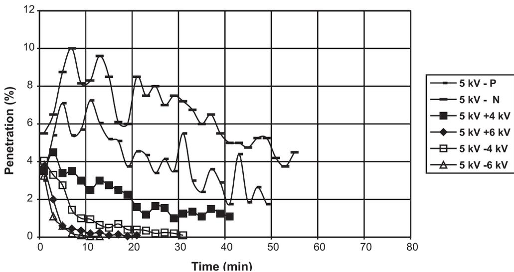
Figure 10. Changes in penetration with time of loading with dolomite dust (as specified by Standard No. PN-EN 143:2004 [10]) such as sampled—P, neutralised—N, ionised with a voltage of  $-4$  kV and  $-6$  kV and with a voltage of  $+4$  kV and  $+6$  kV for a melt-blown polypropylene filter material corona-charged at 5 kV.
