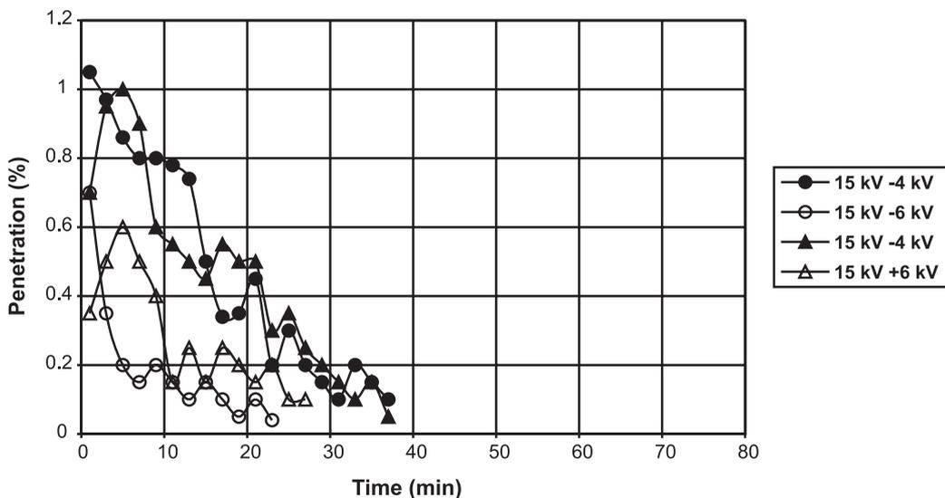
**Figure 8.** Changes in penetration with time of loading with copper-mine dust such as sampled—P, neutralised—N, ionised with a voltage of  $-4$  kV and  $-6$  kV and with a voltage of  $+4$  kV and  $+6$  kV for a melt-blown polypropylene filter material corona-charged at 15 kV.
